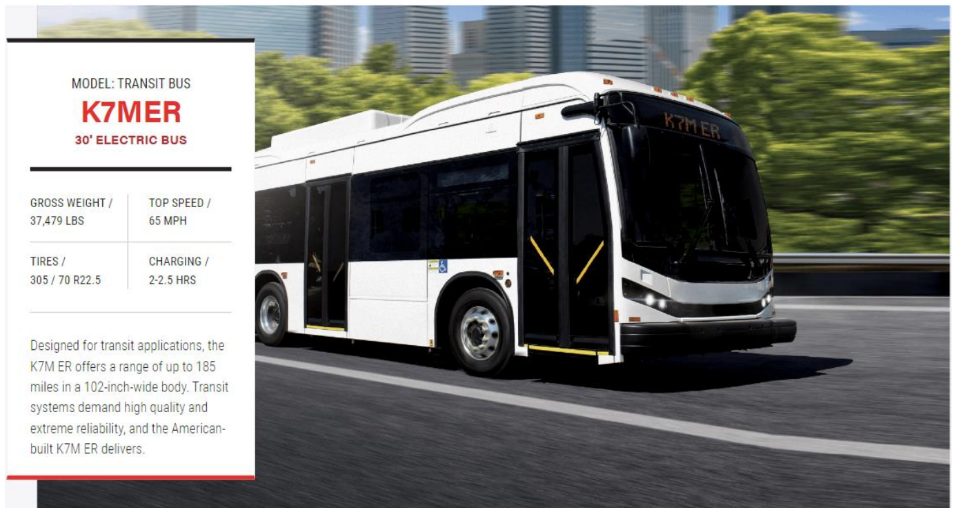
FIGURE 7: ELECTRIC VEHICLE PROTOTYPE EXAMPLE BYD K7MER 30-FOOT ELECTRIC BUS SPECIFICATIONS
